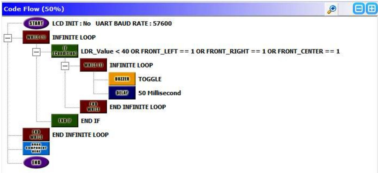
This sample code shows the basic application of sensors and buzzer.
