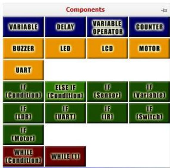
Depending upon the use of the component blocks they are divided in five different categories. Start & End logic blocks are already added to the code flow which indicates start and end of Qu-Bot Program. These blocks can't be dragged from component window.
