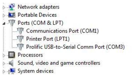
In case of any problem to verify that driver is installed correctly you can check Control Panel-System-Device Manager – Ports. There should be a device called Prolific USB-to-Serial Comm Port (Port number).
